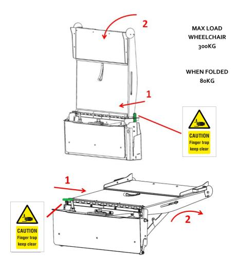
To use the ramp for a wheelchair again, the ramp must be folded up. The ramp will lock itself when folding up. However check carefully whether the ramp is locked to prevent the mechanism from malfunctioning in the future. The ramp is only successfully locked when the locking lever is horizontal and a click is heard.
