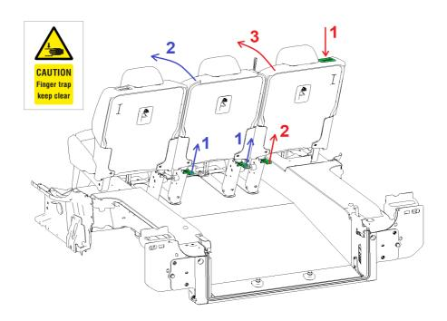
When seats are folded away, extended latches have to be opened manually before folding the seats to seating position. To realize the seating position, follow the steps shown in the picture below. First you have to unlock the seats (1). Then you have to pull the seats backwards (2) till the latches will lock the seats automatically (3).
