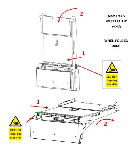
To use the ramp for a wheelchair again, the ramp must be folded up. The ramp will lock itself when folding up. However check carefully whether the ramp is locked to prevent the mechanism from malfunctioning in the future. The ramp is only successfully locked when the locking lever is horizontal and a click is heard.
