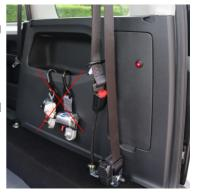
(Re) install both rear retractors on the floor, now they can be mounted and connected to the wheelchair. Knobs on the side of the retractors are used to tighten the belts.
