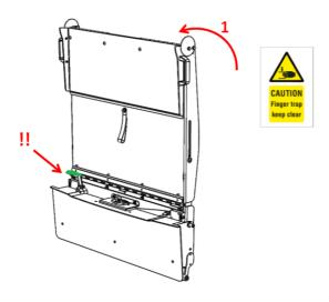
To prevent damaging the ramp it is not allowed to stand on the edges of the ramp when it is being used..
